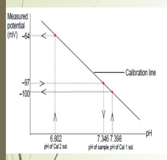
This is a 2-point calibration. In 1-point calibration, only the position of the calibration line is determined. The slope of the calibration line is maintained from the last 2-point calibration.
